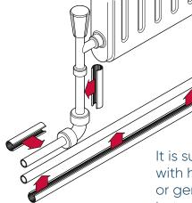
Snappit Cover is compatible with plastic or copper pipe.
