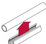
Push the open side of the cover onto the pipe. Snappit Cover will flex and snap into position to grip the pipe.
